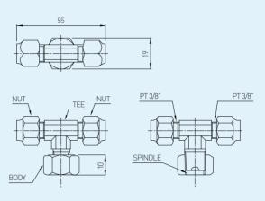
Component actuating Cylinder Valve by Nitrogen gas pressure and located on top of cylinder valve. It functions as same as Needle valve on FM-200 system.
