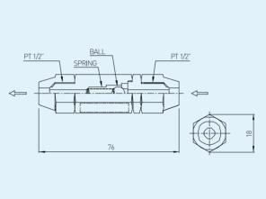
A check valve which keeps CO2 from flowing backward.
