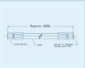
A tube made of rubber. It can substitute copper tube.
