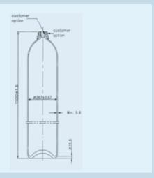
A cylinder for storing CO2 gas at 15.0 Mpa working pressure.
