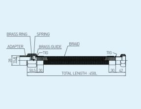
It is located between Cylinder valve and Manifold pipe and comes with check valve which keeps nitrogen gas from flowing backward.
