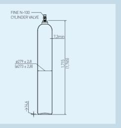
A container for storing compressed gas by pressurizing 22.3 Mpa at at 21°C Agent quantity is  $17.4\,\mathrm{m}^3$
