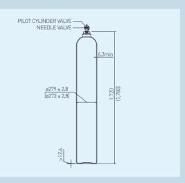
A Cylinder storing 10.0MPa nitrogen gas. It is activate IG-100 cylinder valve by releasing CO2 gas from Actuating Device.
