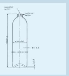
A Mn-Steel container for storing liquefied gas at 15.0 Mpa working pressure. It should be certified by KGS.
