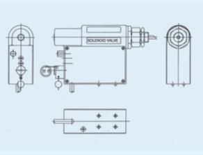
It is an electromechanically operated valve. It activates CO2 cylinder valve in actuating device
