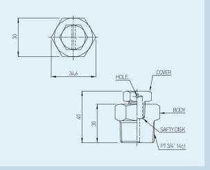
A valve which automatically releases gas agent when the pressure exceeds preset limits. It prevents manifold broke down.
