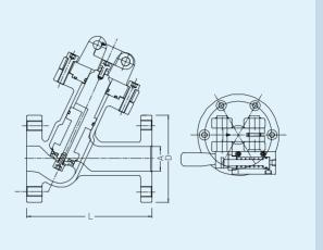
A valve discharges gas agent selectively to where it is needed if you need to make single manifold with more than two Enclosure.
