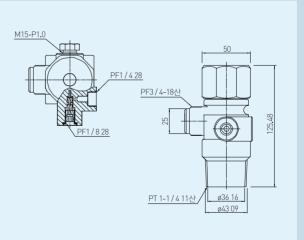
It is a valve used to control the timing and quantity of gas flow into an engine. It functions with 9 Mpa regulating pressure at 21  $^{\circ}\text{C}$
