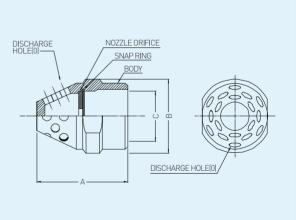
A Nozzle to discharge gas agent to Enclosure effectively, making agent quantity and timing on time.
