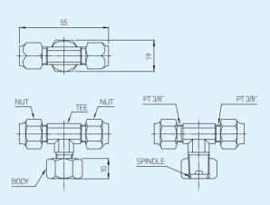
A valve used to control gas agent discharge mistakenly when CO2 cylinder leaks.
