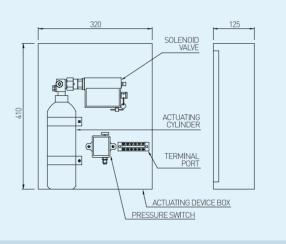
Activating device to release high pressured gas from CO2 cylinder by using solenoid valve. The discharged gas opens selection valve and cylinder valve.
