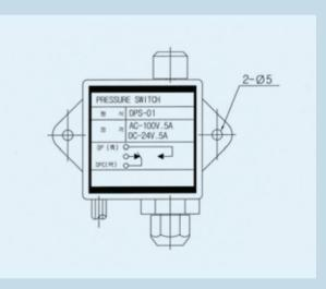
A devive to turn on the discharge Lamp, it is activated by outlet gas pressure.
