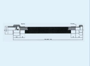
A hose to connect between cylinder and manifold to deliver gas agent from cylinder, coming with check valve.
